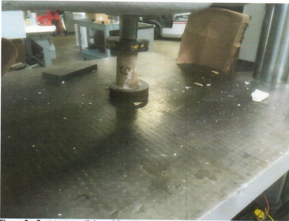
Figure 2. Post test condition of Specimen #2 - typical break.
