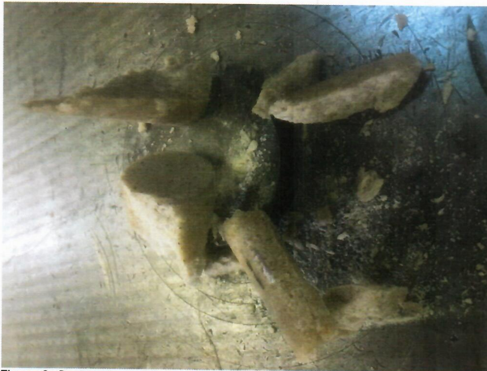
Figure 3. Post test condition of Specimen #11 - also typical.
